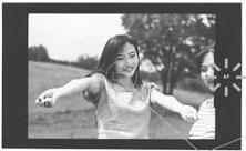
(Make sure) Autofocus frame The autofocus beep is heard, and the autofocus indicator lights in the viewfinder. 2 Reposition your subjects in the picture frame while keeping the shutter release button depressed halfway. Then press the shutter release button fully.
