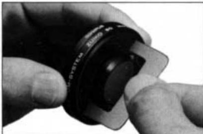
If it is hard to unscrew the close-up lens, use a wrench provided.
